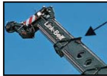
A-max extends only the inner-mid section of the boom for substantially increased capacities for in-close, maximum capacity lifts.
