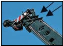
A-max extends only the inner-mid section of the boom for substantially increased capacities for in-close, maximum capacity lifts.
