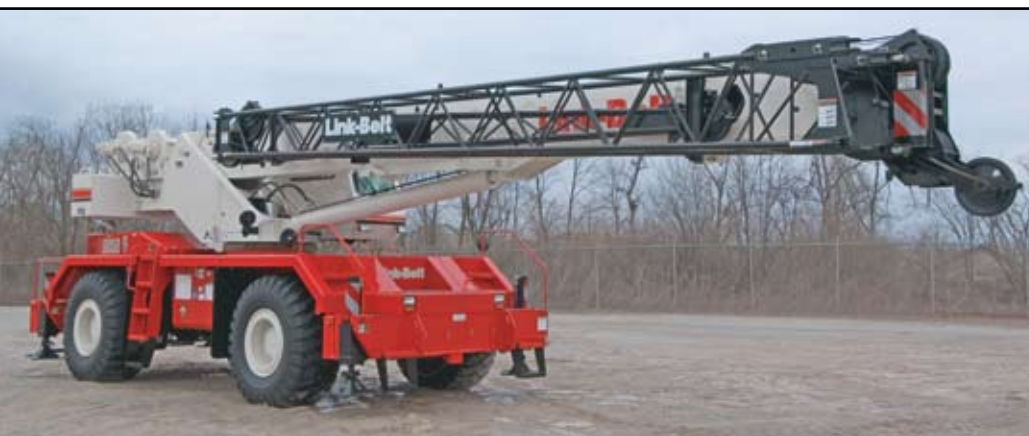
A-max extends only the inner-mid section of the boom for substantially increased capacities for in-close, maximum capacity lifts.
